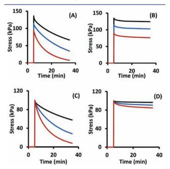
**Figure 3.** Stress relaxation profiles of the controls and real samples loaded with various levels of the Ru catalyst (black line, 0.0050 mol %; blue line, 0.0075 mol %; red line, 0.010 mol %). (A,C) samples with catalyst; (B,D) controls. (A,B) constant strain; (C,D) constant initial stress. The strain or stress was applied at t = 5 min and the relaxation was conducted for 30 min.
