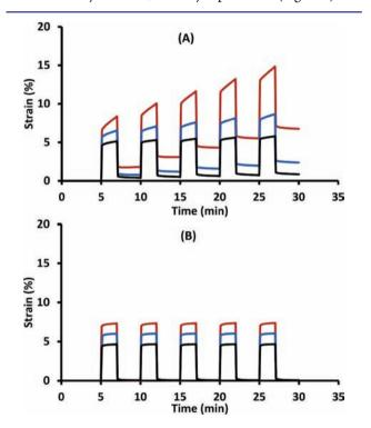
**Figure 2.** Cyclic strain/recovery profiles of the controls and real samples loaded with various levels of the Ru catalyst (black line, 0.0050 mol %; blue line, 0.0075 mol %; red line, 0.010 mol %). The force was alternated between 1 N for 2 min and 0 N for 3 min from t = 5 min to t = 30 min. (A) Samples with catalyst; (B) controls.
