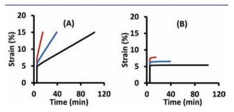
**Figure 1.** Strain profiles of the controls and real samples loaded with various levels of the Ru catalyst (black line, 0.0050 mol %; blue line, 0.0075 mol %; red line, 0.010 mol %). (A) for samples with catalyst, 1 N of force was applied from t = 5 min until the strain reached 15%. (B) for controls, 1 N of force was applied from t = 5 min for the same time as the corresponding samples with catalyst.
